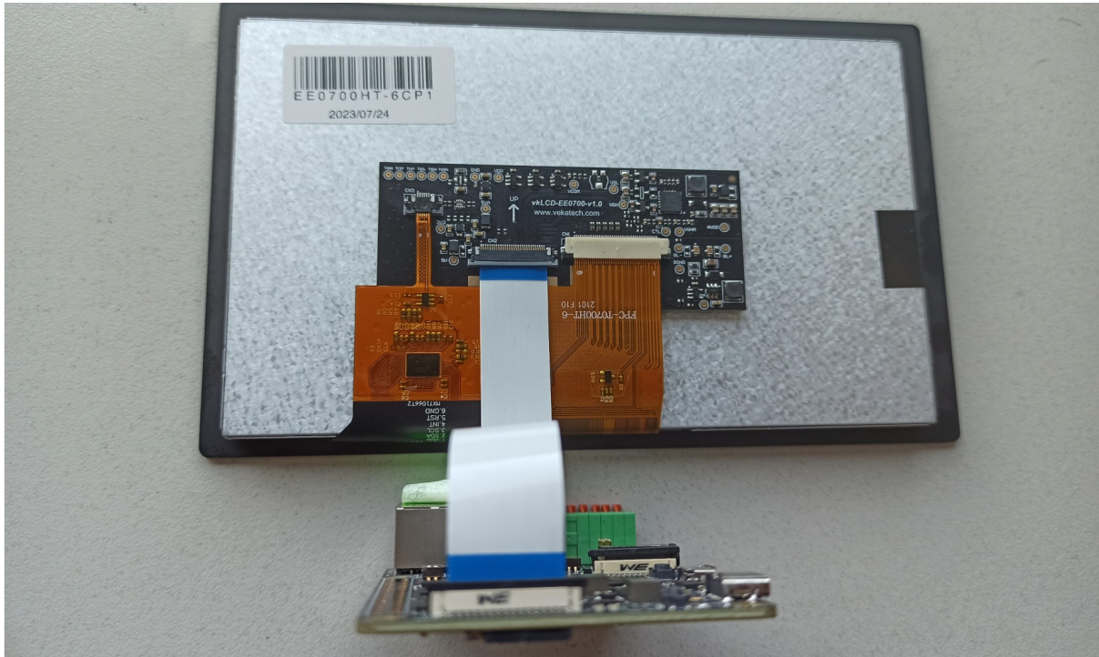
vkcz-dsi-vklcd-ee0700 display FPC cable orientation
